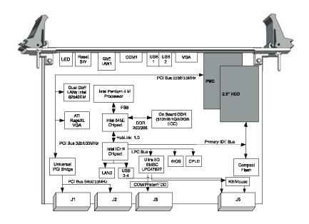
Figure 1.1: MIC-3358 functional block diagram.
